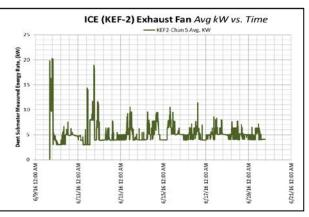
Location: ICE, NY, NY. Data taken from 6/9/2016-6/27/2016. Submeter (3) Dent ElitePro. Heat/yr 8,161,253,000, BTU/yr — NickleFisher \$/kWh \$0.18. Cool/yr 512,942,000, BTU/yr — NickleFisher \$/Therm \$0.95. 343 Days/yr. 24 hrs/day, Cooling Set point 72F, Heating Set point 68F.
